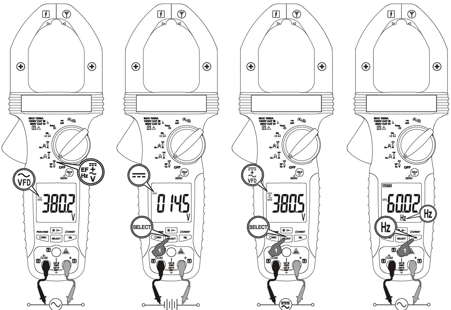
Note: **ACV** (and hence **AC+DCV** & **Line-level Hz**) function is equipped with digital low-pass filter, and is capable of dealing with **VFD** (Variable Frequency Drives) signals. It also improves ACV reading stability in noisy electrical environments.
