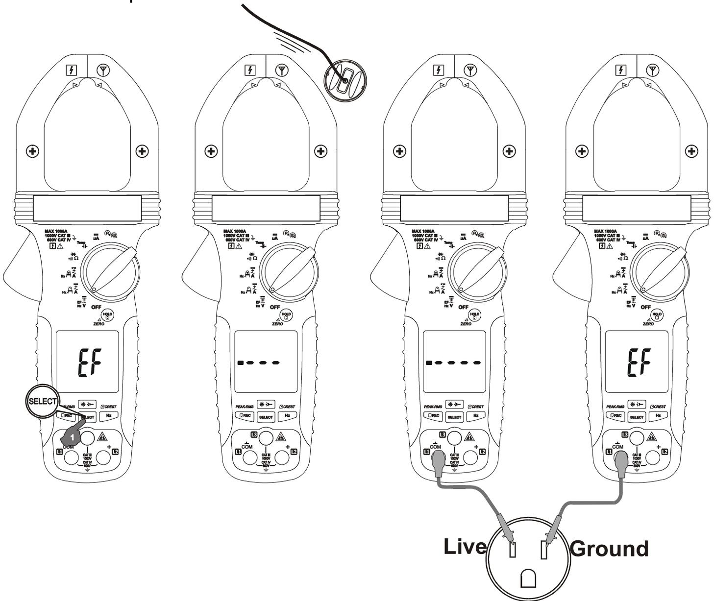
● **Non-Contact EF-Detection:** An antenna is located along the top-right end of the stationary clamp jaw, which detects electric field surrounds energized conductors. It is ideal for tracing live wiring connections, locating wiring breakage and to distinguish between live or earth connections.
