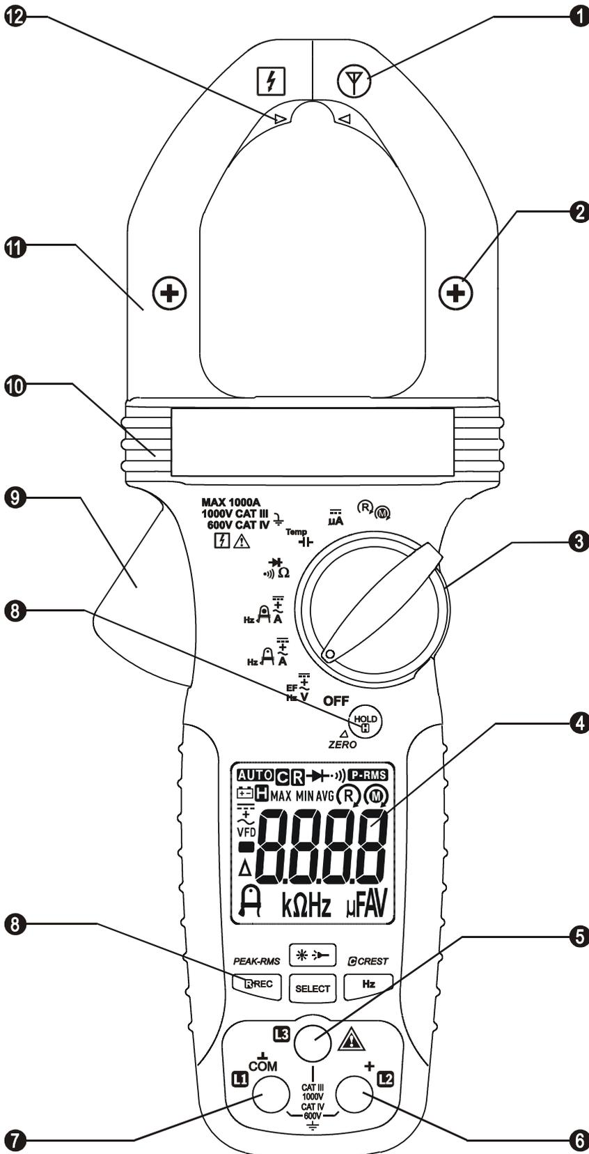
1) Antenna area for Non-Contact EF-Detection
