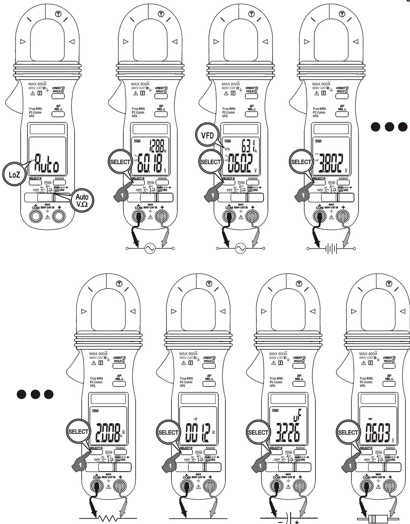
While in AutoCheck™ function, press SELECT button momentarily to manually select the low input impedance (LoZ) **ACV<sup>Hz</sup>**, **VFD ACV<sup>Hz</sup>** and **DCV** functions as well as the **Ω Resistance**, **•) Continuity**, **⚡ Capacitance** and **⚡ Diode** functions in
