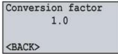
*Fig. 7.2.2 – Screen of setting of voltage conversion ratio*
