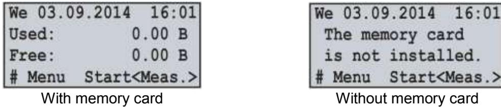
**Fig. 6.2** – Main screen view (with and without memory card)
