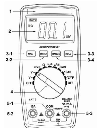
3.3.HOLD (Data Hold): Press the button, the reading is locked, press the button again, the lock is cleared.
